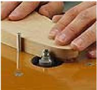
If you're using a piloted bit to rout an irregular-shaped work piece, the beginning of a cut can be a bit tricky. That's because the bit has a tendency to grab the work piece.
