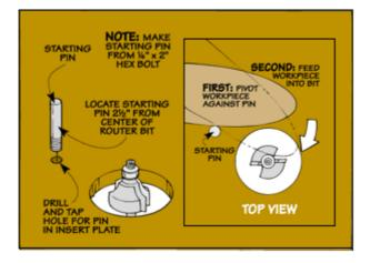
It's easy to use a starting pin. Simply pivot the work piece against the pin as you feed it into the bit. The pin provides the leverage needed to make a controlled cut.
